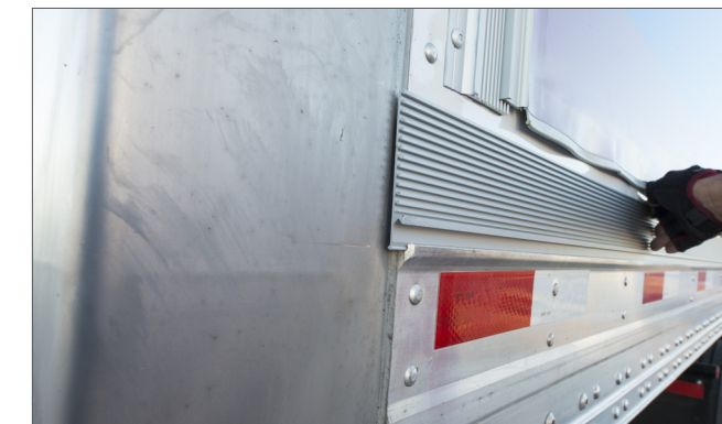
FRAME SLIDING INTO THE BOTTOM TRAILER RAIL
